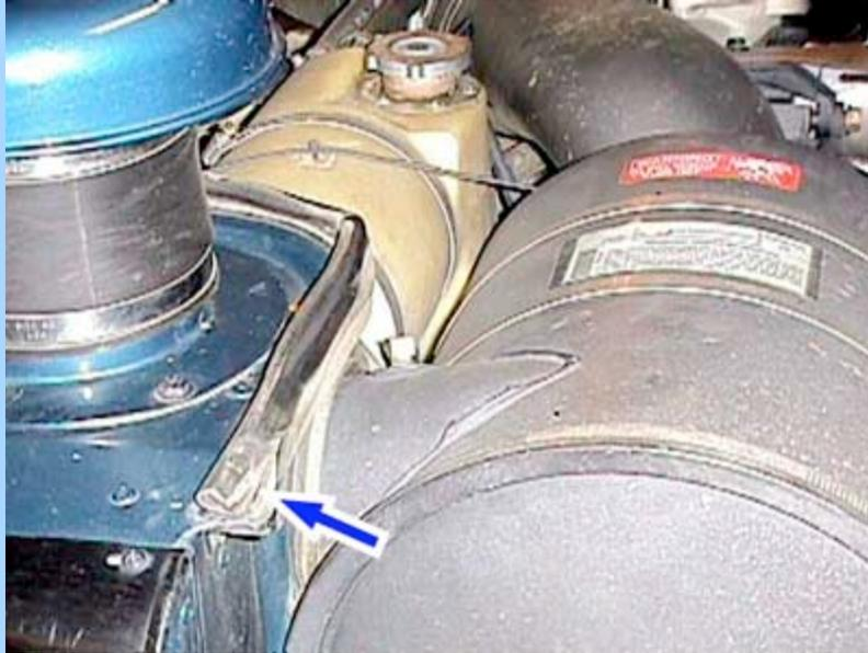
The rubber piece on the hood was added sometime in the 1993 or 1994 model year. Its purpose is to deflect water (from a bow wave sweeping up over the hood) away from the air intake. The LE trucks and some 1993 trucks do not have this piece.
