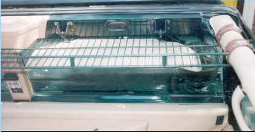
window. I put felt under the hose clamps to prevent damage from the sharp edges of the clamps. Reinstall the visors, they will fit right through the rack. If extra support is needed there are holes in the underside of the windshield frame where you can install cable guides to stabilize the rear of the rack. I did not find it necessary as there was not much flex in the rack
